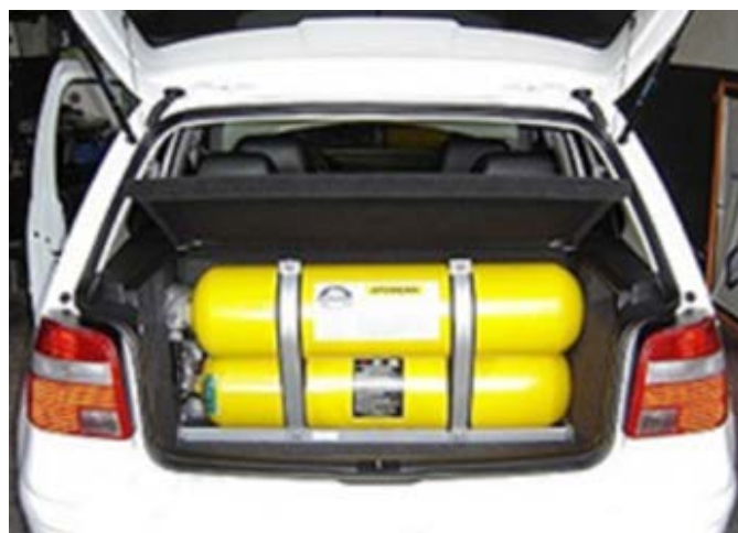
Fig. 5: A CNG retrofitted vehicle
